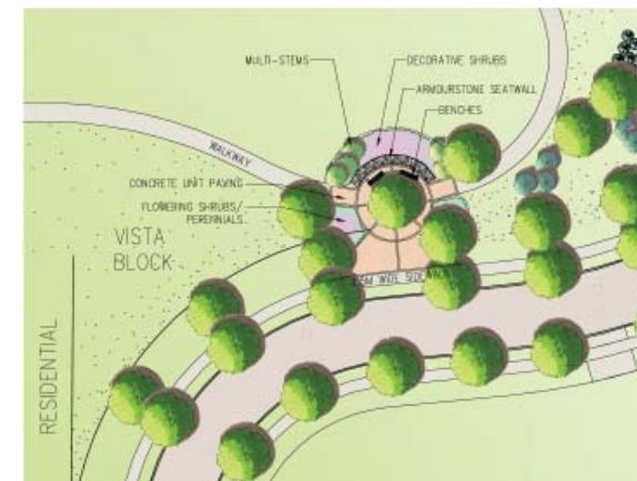
Figure 5.4d - Vista Block Typical Entry Demonstration Plan
